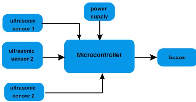
Figure 2. Block Diagram of Overflow Control Mechanism
