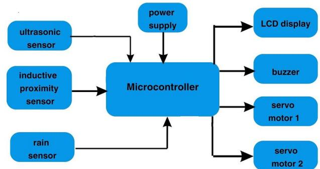
Figure 1. Block Diagram of Smart Waste Segregator
