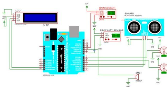
Figure 3. Wiring Diagram of Waste Segregator
