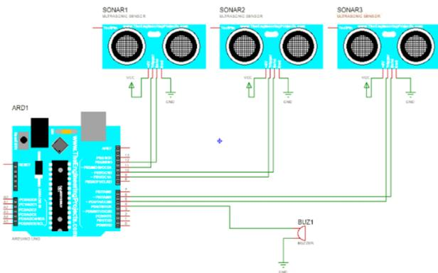
Figure 4. Wiring Diagram of Overflow Control
