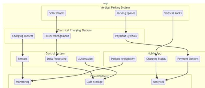
Block diagram of the Smart vertical parking system Challenges
